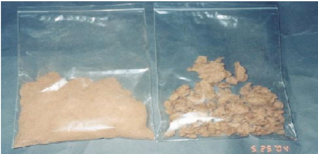
Fig. 2. Fibres from two cycles (2.5-mm plate gap followed by 0.5-mm) of refining (left) and Lumpy fibres from one cycle (0.5-mm plate gap) of refining
